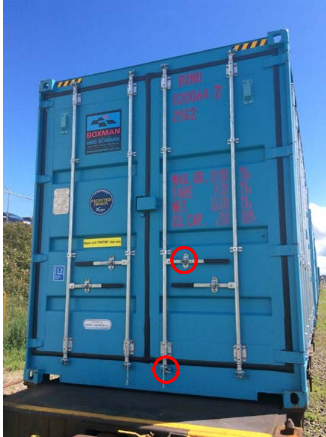
1 seal, in EITHER circled location is required
