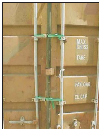
Doors secured using correct strap and buckle.
